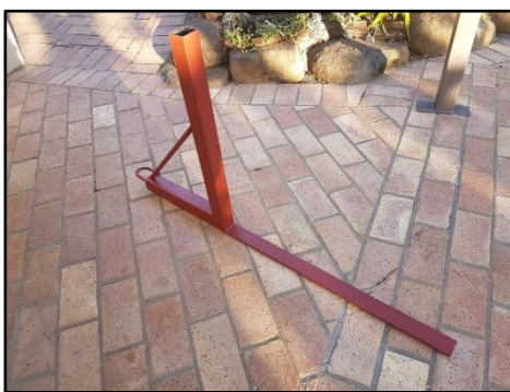
Formwork support brackets
